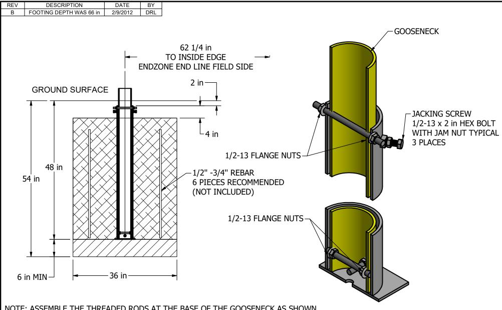
NOTE: ASSEMBLE THE THREADED RODS AT THE BASE OF THE GOOSENECK AS SHOWN, PLUMB THE GOOSENECK WITH THE THREE JACKING SCREWS AT THE TOP OF THE SLEEVE BEFORE CROSS DRILLING THROUGH THE SLEEVE AND MAST AND ASSEMBLING THE 8 in THREADED ROD AND NUTS AS SHOWN
